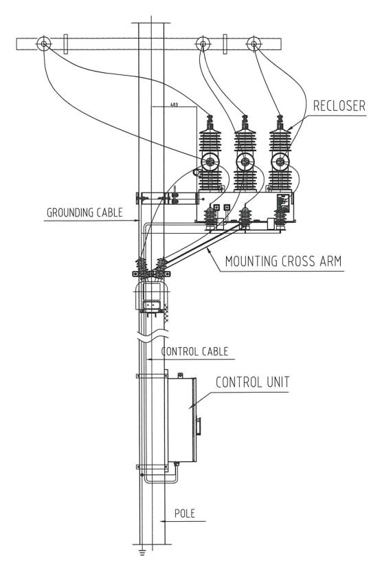
Note: Voltage transformers, surge arresters are out of supply scope
